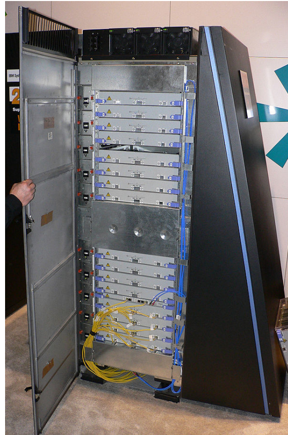
A Blue Gene/L cabinet showing the stacked blades, each holding many processors
