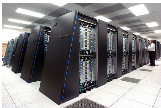
The Blue Gene/P supercomputer at Argonne National Lab runs over 250,000 processors using normal data center air conditioning, grouped in 72 racks/cabinets connected by a high-speed optical network [1]
